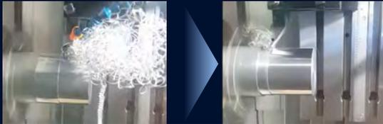
**Comparison of results between regular turning operations and CBS machining**
